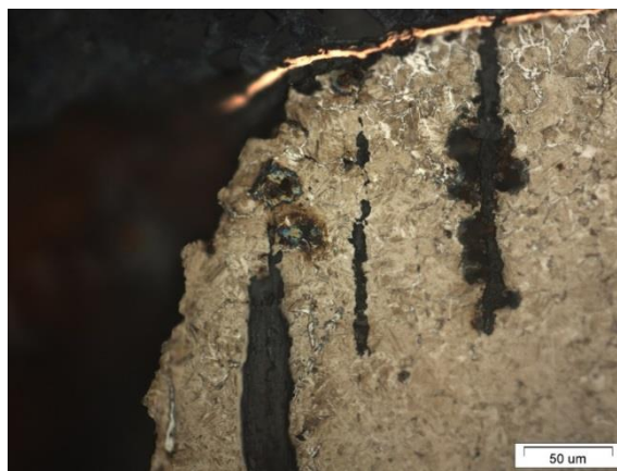
Fig. 3. Microstructure of the corrosion center of wheel lock
