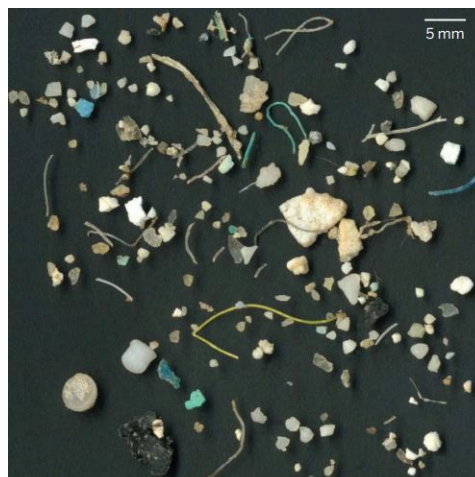
Fig. 3. Microplastics collected in North Pacific subtropical gyre with a surface plankton net
