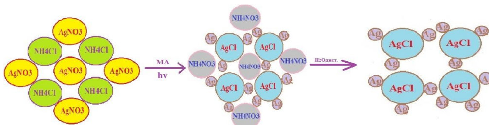
Fig. 2. The reaction mechanism of the process of mechanochemical activation
